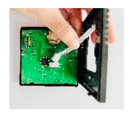
Finally, carefully clip the front part to the rear housing. It can be opened again later using the tabs if necessary.
